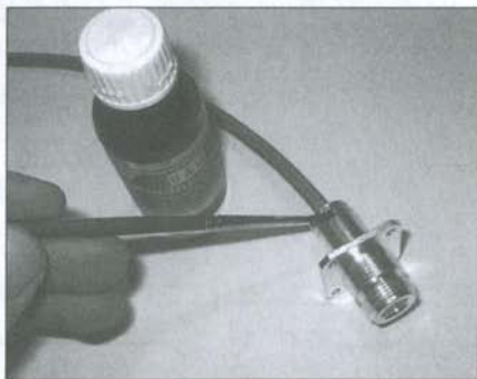
Fig. 7: Sealing the N connector with fishing rod varnish
