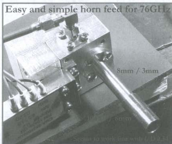
Fig. 10: Simple 76GHz horn feed for use with the Fresnel lens
