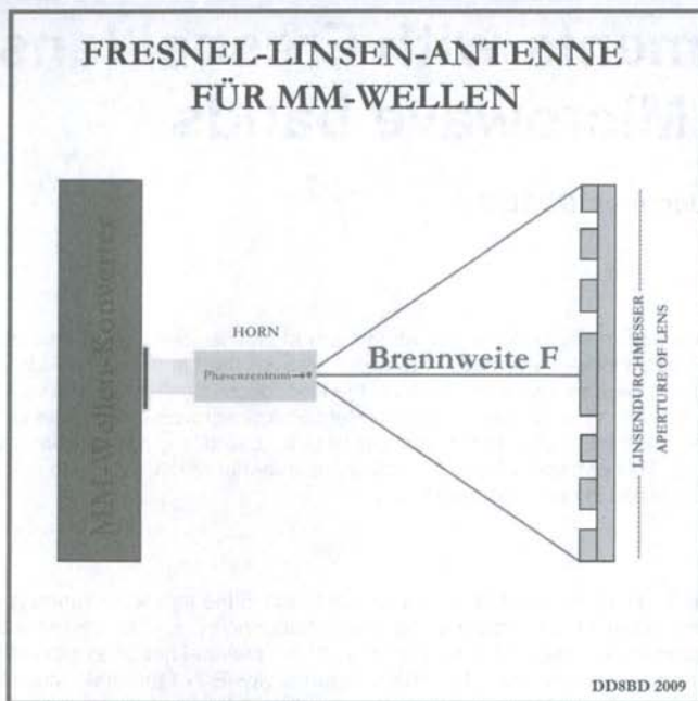
Fig. 1: Using a Fresnel lens as part of a mm-wave antenna
